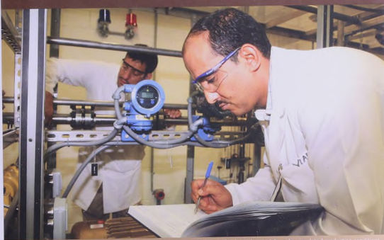
The company's downstream research projects include studying the performance of industrial materials under simulated production conditions. Here, company researchers monitor the progress of a corrosion simulation experiment utilizing a unique corrosion flow loop apparatus.
