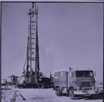
In this Schlumberger vehicle are special instruments which record the data taken from the well and convert it into readable form.
