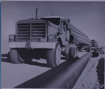
A huge truck, driven by Khalifah Muhammad, carries 80-foot, 24-ton lengths of pipe for the Safaniya pipeline.
