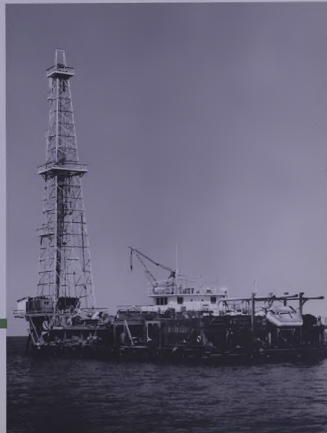
Safaniya plans call for the drilling of additional offshore wells by the Company's drilling barge.
