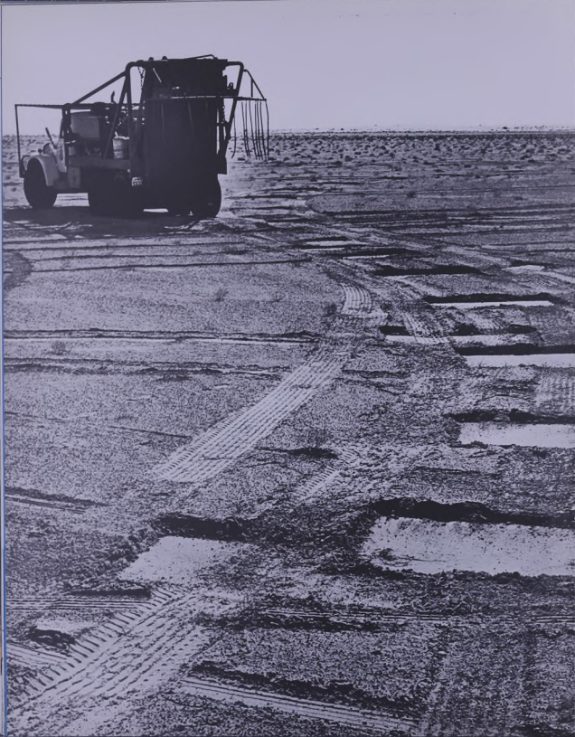
A seismic exploration device new to Saudi Arabia, the geograph thumps across desert terrain.
