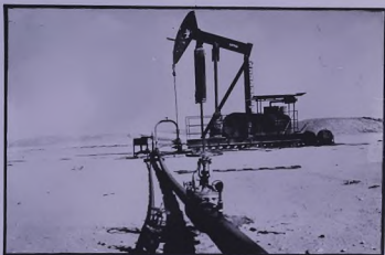
The earlier acquired air balanced model can be distinguished quite easily from the new crank balanced pumping units.
