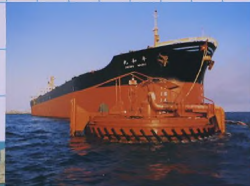
Oil is loaded for export to world markets by means of a Single Buoy Mooring (smb) and two fixed tanker berths
