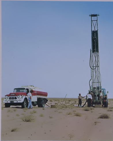
A seismic party engaged on shot-hole drilling
