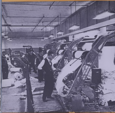
Printing machine — materials are printed with fast dyes and in designs prepared at the factory.
