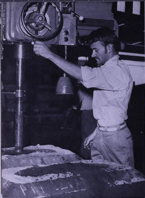
Taking a core sample from an Alba manufactured anode block with a drilling machine and a diamond core drill.
