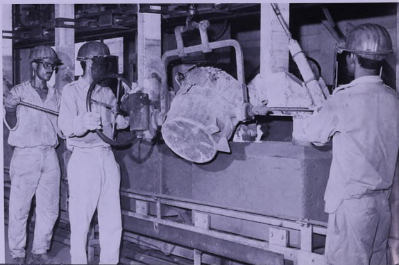
Sealing a Rod into an anode, using molten cast iron.
