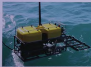
The Remotely Operated Vehicle is deployed to inspect underwater pipelines and infrastructure, while satellites are used to facilitate communications.
