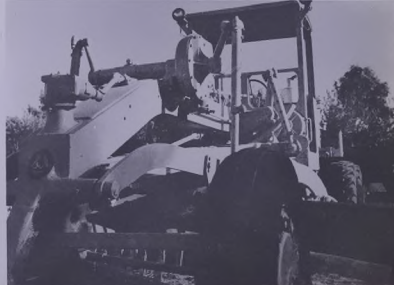
A machine for levelling roads, run-ways and landing strips.
