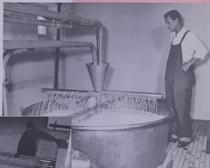
The bleaching operation that turns cotton snow-white.
