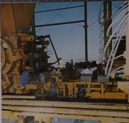
A section of the Besser V3-12 Vibrapac block-making machine.
