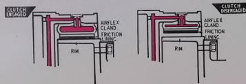
Illustration left shows Compressed Air Admitted to Airflex Gland Engaging Clutch. Illustration right shows Air Released. Note large clearance between Rim and Slippers.
