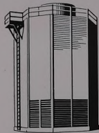
Fluor "Counterflo" induced draft cooling towers, prefabricated in mass production, come in multiple or single cells, any size or height.
