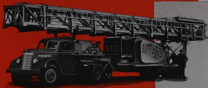
Ideco "Rambler Rig" consisting of a Kwik-Lift Mast with Hydraulic Hoist.
