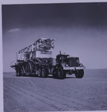
The mobile T-20 structure drilling rig can be moved efficiently to locations in remote areas.
