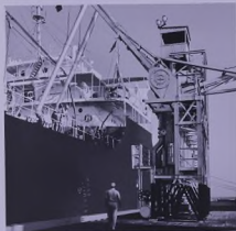
Mechanical loading arms speed pier operations.
