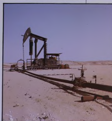
More than seventy of these turbin pumps will be installed at Marmul and in the nearby fields.
