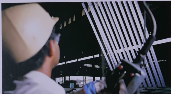
Lifting extrusion billets from the Direct Chill (DC) Caster
