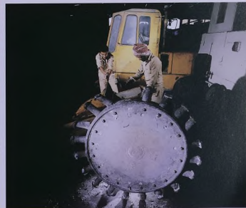
Repairing a crusher in the workshops
