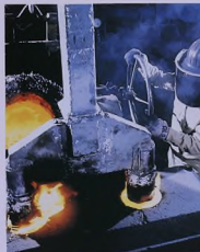
Sealing a rod to an anode
