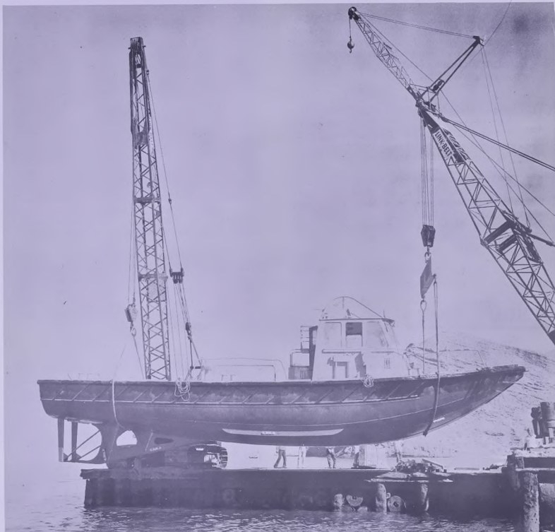
The mooring launch SIYMA being refloated after her two year refit. This is the first time that a mooring launch of this size has been slipped at Mina al-Fahal.
